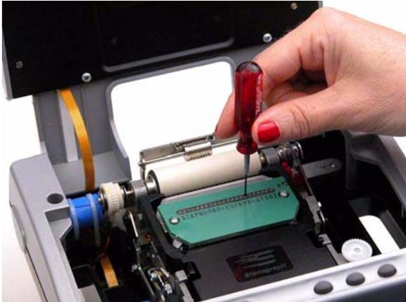
Adjust the number bar contact only when all your number settings are either too heavy or too light. To adjust an individual number, adjust the contact of the corresponding letter for that number. For example, to adjust the number 8, adjust the key contact for the final L. By adjusting the number 8, you also adjust the letter L.
