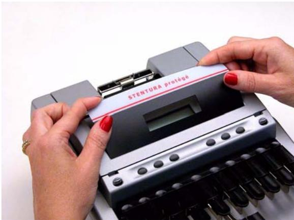
3. Push on the top gently to slightly bow the nameplate and insert the top into the top of the nameplate frame.
