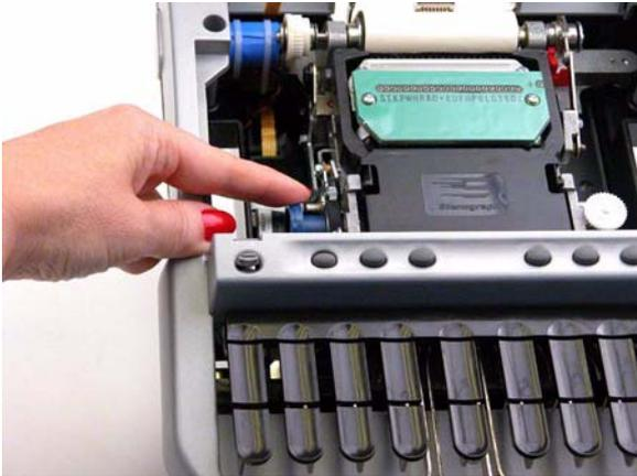
3. Turn the knob towards the front of the Stentura Protégé as indicated by the arrowheads on the rim of the knob. You should only turn this knob toward the front of the steno machine.
