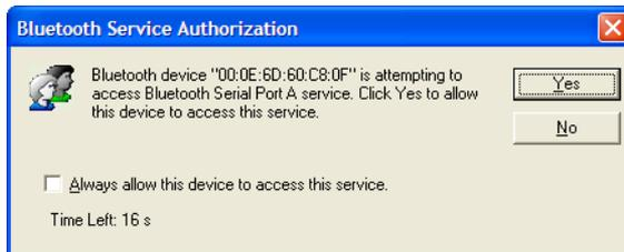
You have 30 seconds to respond to this dialog box. If you do not press **Enter (Yes)** within 30 seconds, you must disconnect the Socket Cordless Serial Adapter from the Mira/fusion and reconnect it to redisplay the Enter Bluetooth Passkey dialog box and enter the Passkey code.
