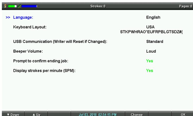
2. Touch the **Up/Down** sensors as necessary to highlight the Display Strokes per minute (SPM) option.
