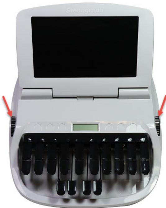
The depth of stroke adjustment wheel, on the left, determines the height of the number bar and all the steno keys. This affects how far the keys go down when you press them. There are ten different positions for the keyboard.
